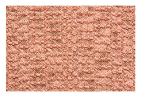
Blocks are often repeated with plain weave in between. Plain weave can be woven across and down the length of the fabric. The drawdown below shows the possible options. The fabic is a sampler showing various arrangements of the blocks.
